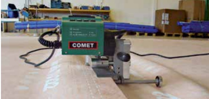
Hands-free welding due to integrated guiding plates.
