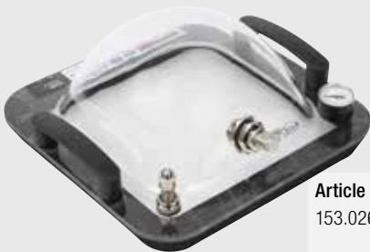
For testing T-joints
