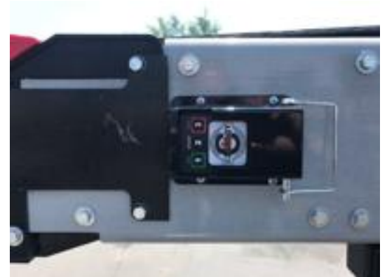
Fig. 3-2 Control valve at nose of EXT-52 conveyor allows receiving person to control material flow.
