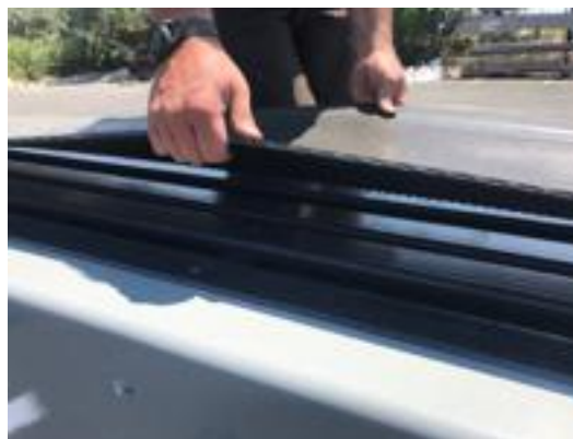
Fig 4-2 Conveyor belt tension is correct when belt can be lifted 4-6 inches in middle on conveyor.
