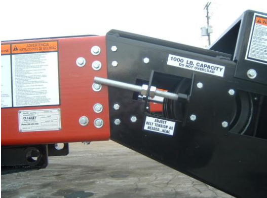
Fig 4-3 Conveyor belt tension is adjusted by turning the adjusting screws at the base at the end of the conveyor.
