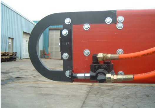
Fig. 3-2 Control valve at nose of FBR conveyor allows receiving person to control material flow.
